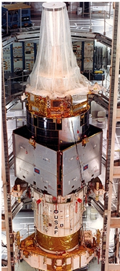
Defense Support Program satellite atop an Inertial upper Stage prior to launch. (NASA photo)
