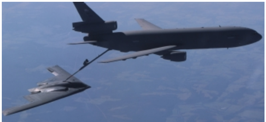
B-2 Spirit being refueled by a KC-10 A Extender (USAF photo by Gary Ell)
